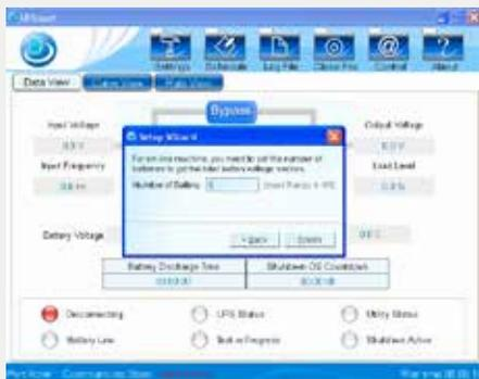
3.- Setup number of battery: The number of battery must make sure correct ,in order to the software can automatically calculate to obtain relevant information of the battery. Set the battery and then click the finish button, the software can automatically connect the UPS.
