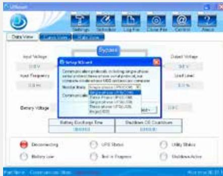
2.- Quickly set up monitoring mode and the communication port, as follow figure.
